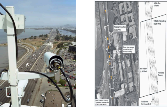
Figure 18: Left picture shows a digital video camera mounted on top of a building that overlooks I-80. Right one is the aerial photograph of the extent of the I-80 study area.
