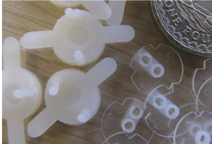
Figure 13. Runner systems compared to replicated parts
