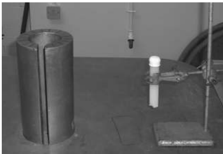
Figure 5.4: Polymerisation of rods in gamma radiation source
