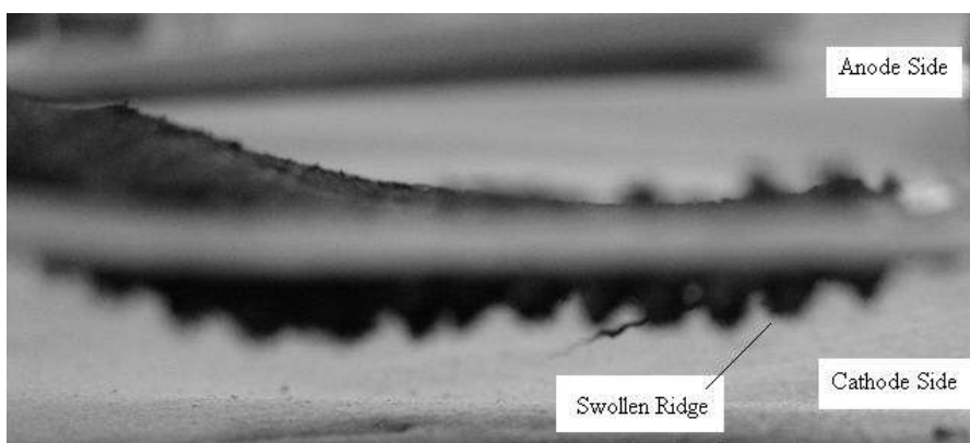
Figure 6.27: 06SJG038O MEA after cell testing
