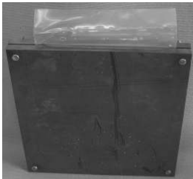
Figure 5.6: Brass plates used for thermal polymerisation of membranes
