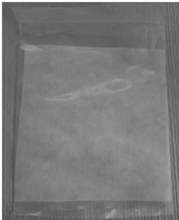
Figure 5.5: Solution soaked separator prior to thermal polymerisation
