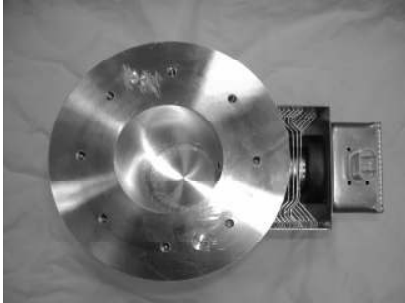
Figure B.4: Photograph of the finished single-mode cavity with magnetron fitted (cavity size; radius 3.375 cm, length 17.00 cm).
