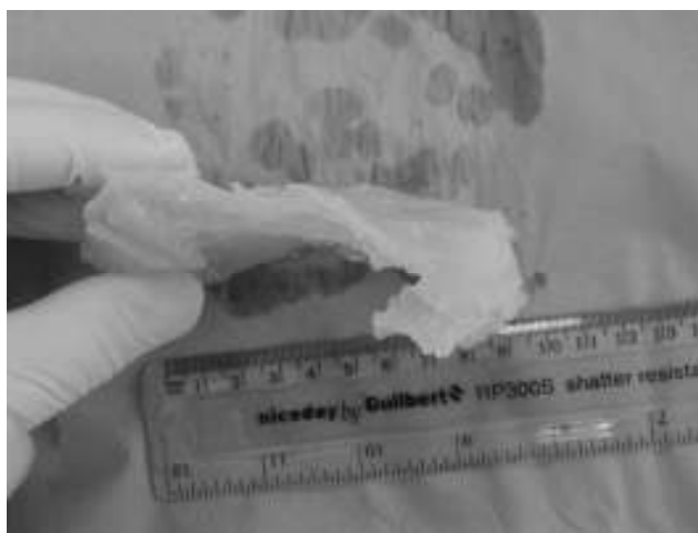
Figure 6.39: Sample showing break-up of membrane due to physical stress after hydration
