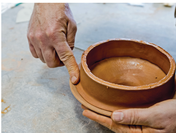
Figure 4: While the mold provided the necessary firmness, the vertical wall was built on it by adding, fixing, pinching and smearing of several clay coils (© V. Brigola).
