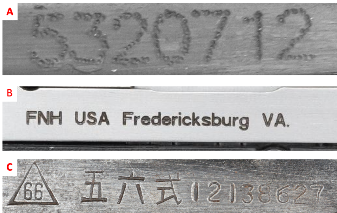
Figure 2-5: Three methods of serial number and mark application. (A) Dot peening, (B) Laser engraving, (C) Stamping. All photographs courtesy of Conflict Armament Research.
