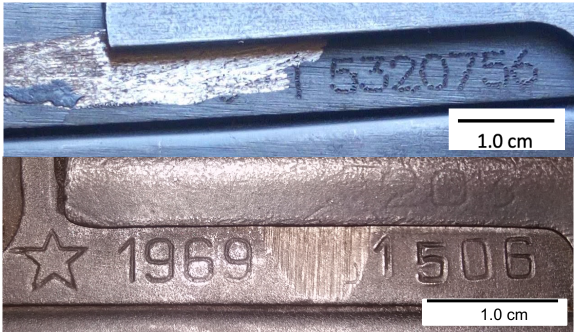
Figure 1: Two examples of the types of photographs examined. A Type 56-1 (top) and an AKM rifle (bottom), both showing partial obliterations.
