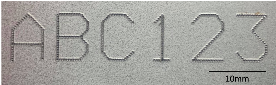
Figure 3-4: A sample of a dot-peened steel plate (size 60mm x 100mm x 2mm).
