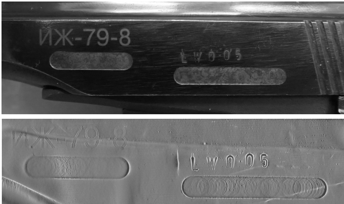
Figure 3-15: The electromagnetic image (bottom) resulting from the ECK scan, showing two milled areas with no discernable marks underneath, a clearly visible stamped mark (LW005) and a faint laser-engraved mark (ИЖ-79-8). The scan was not altered from original using any computer software. (Figure not to scale)
