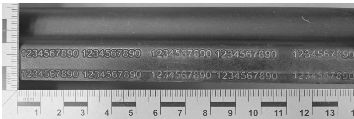
Figure 3-11: The left side of an AK-pattern rifle top cover, with ten laser engraved marks (“1234567890”).
