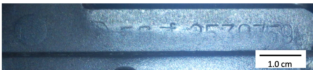
Figure 6: An example of a Type 56 rifle where the top cover would have protected the upper half of the digits and natural abrasion of the surface resulted in the passive removal of the bottom half of the digits.
