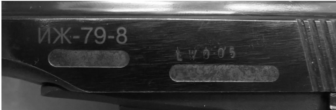
Figure 3-6: A Baikal pistol slide (left profile), showing one visible original laser engraved mark (ИЖ-79-8), one stamped mark (LW005) applied by the LWW, and two regions where milling marks are evident, hiding two additional laser engraved marks.
