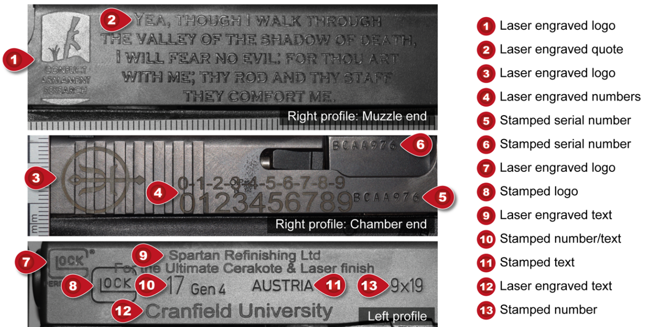
Figure 3-10: The laser engraved and stamped marks removed from the right profile (top, middle) and left profile (bottom) sides of the pistol slide.
