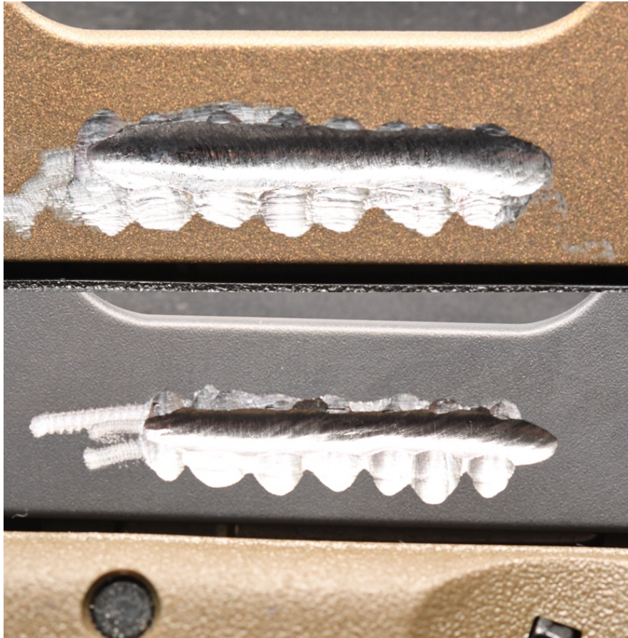
Figure 9-1: Two pistols with the same obliteration code showing the serial numbers removed by a rotary tool moving both left to right and downward with no additional concealment.
