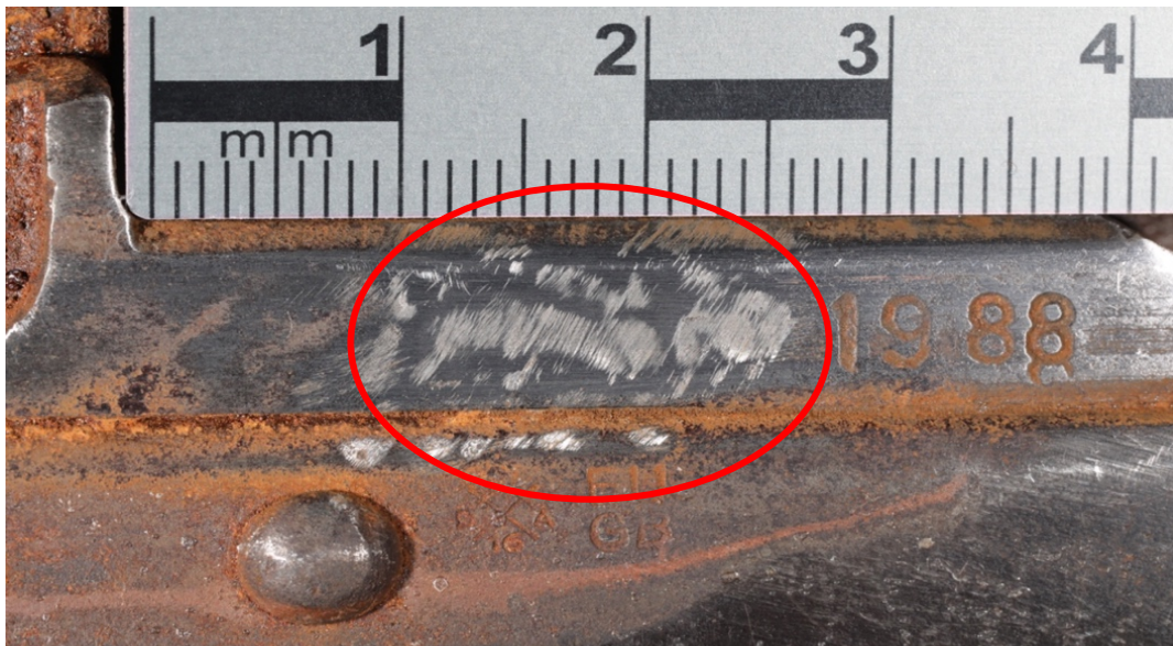
Figure 3-8: An AK-pattern rifle, showing an area of obliteration, where a portion of the serial number was removed (circled).
