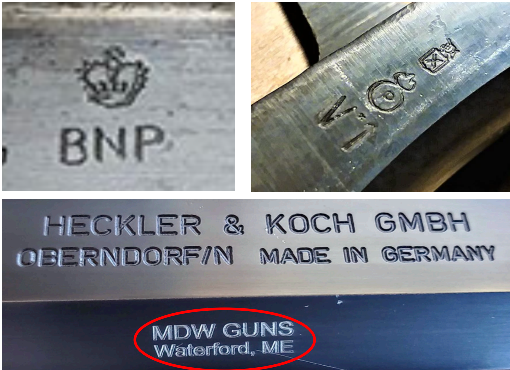
Figure 2-3: Examples of proof marks (top left)(authors own image), inspection marks (top right) [33], and import marks (bottom) [33].
