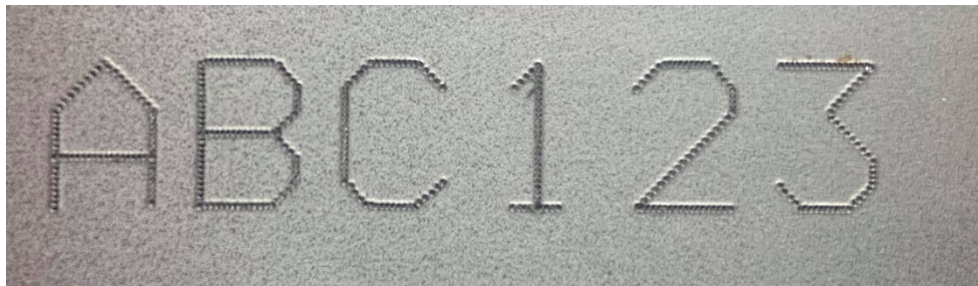
Figure 4. A sample of a dot-peened steel plate (size 60mm x 100mm x 2mm).
