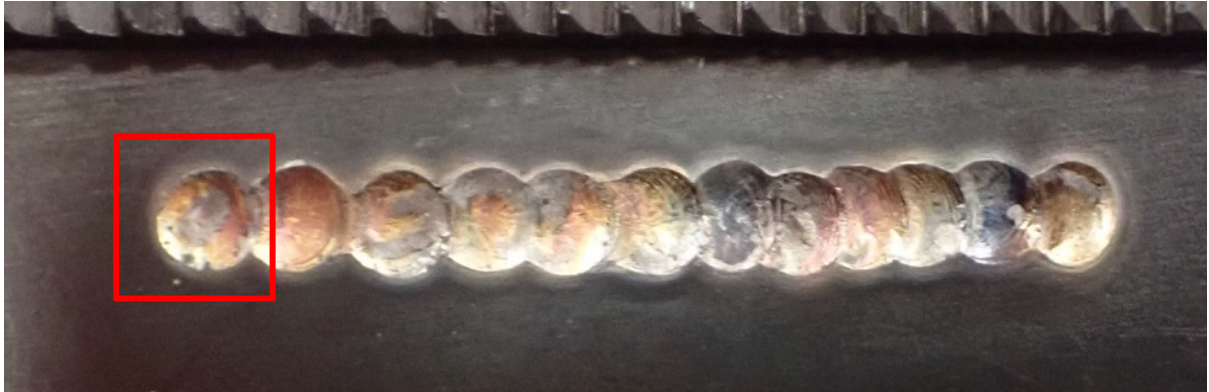
Figure 4-5: An example obliteration where the direction of travel from right to left is indicated by the overlapping toolmarks created as the welding stick is moved across the surface of the firearm.
