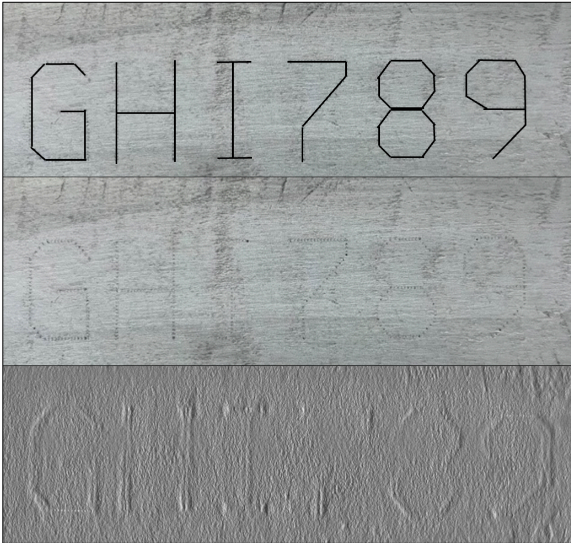
Figure 3-14: The top image shows the characters visible before obliteration. Traditional recovery using Fry's Reagent (middle) and the non-destructive recovery using the ECK (bottom). Both results show "GHI789", showing a complete recovery of all 6 digits. These results have not been filtered, processed, or altered using any computer software. (Figure not to scale)
