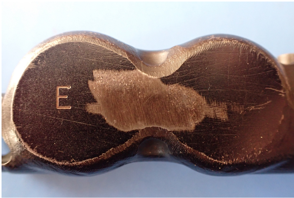
Figure 3-9: The muzzle device of a rifle with a criminal obliteration.
