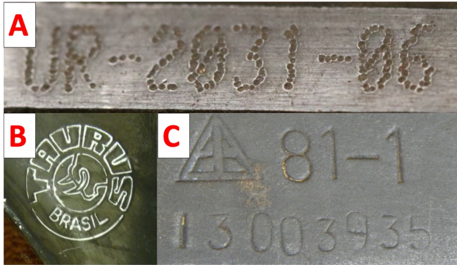
Figure 1. Three methods of serial number and mark application. (A) Dot peening, (B) Laser engraving, (C) Stamping. All photographs courtesy of Conflict Armament Research.
