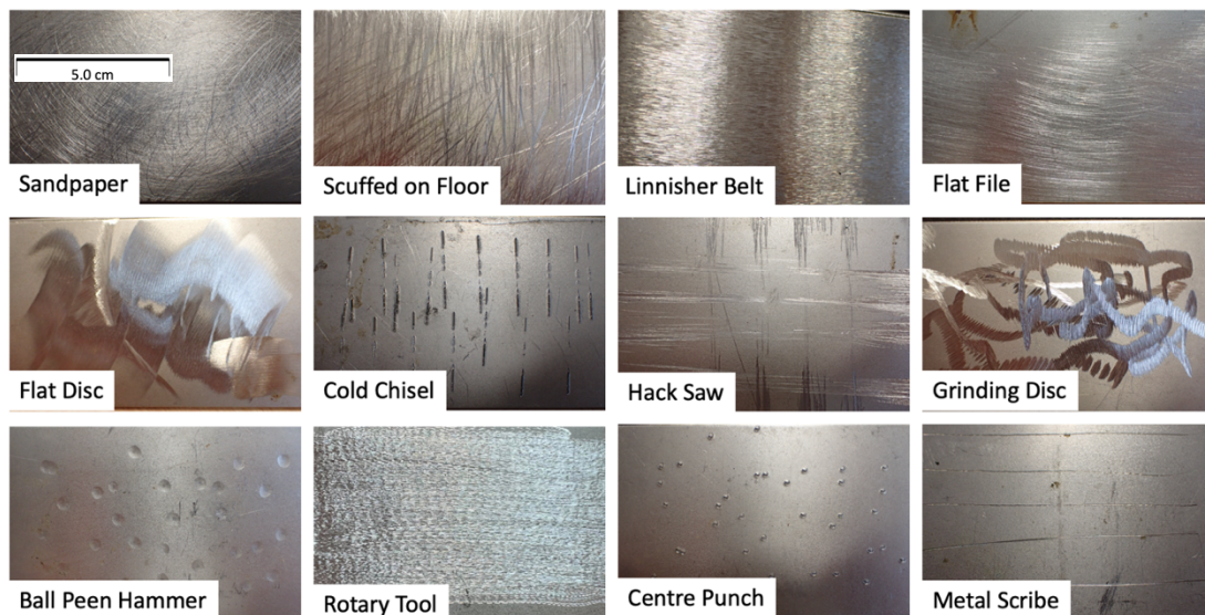
Figure 2: Twelve sample plates showing toolmarks from typical workshop tools to differentiate the various class characteristics to aid the identification of the tool used in an obliteration.
