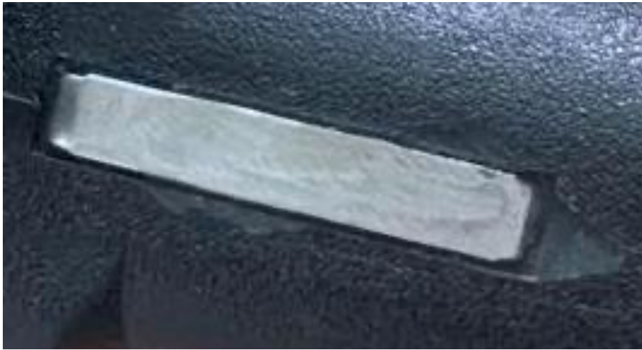
Figure 3-7: The obliterated steel plate that houses the serial number for a polymer-framed pistol.
