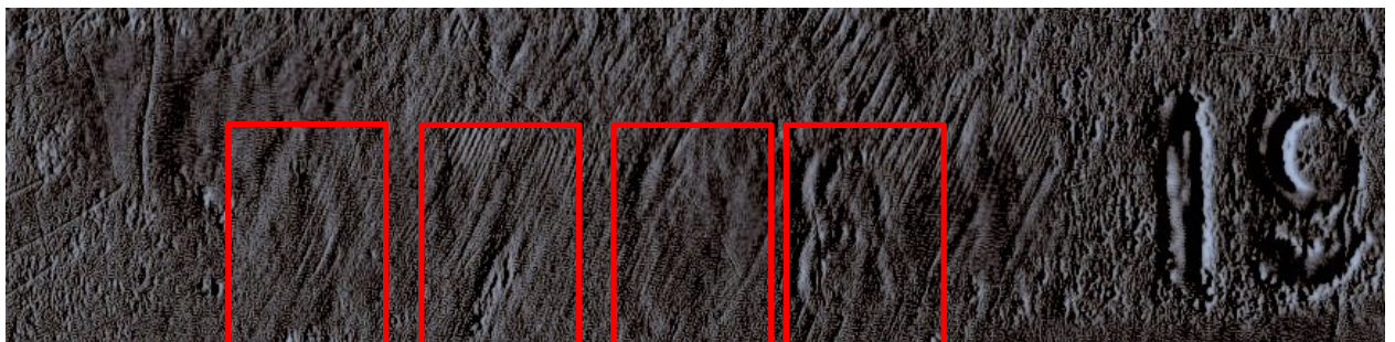
Figure 3-17: "2788" (boxes) recovered in the electromagnetic image of the AK-pattern rifle. Image authors own. (Figure not to scale)
