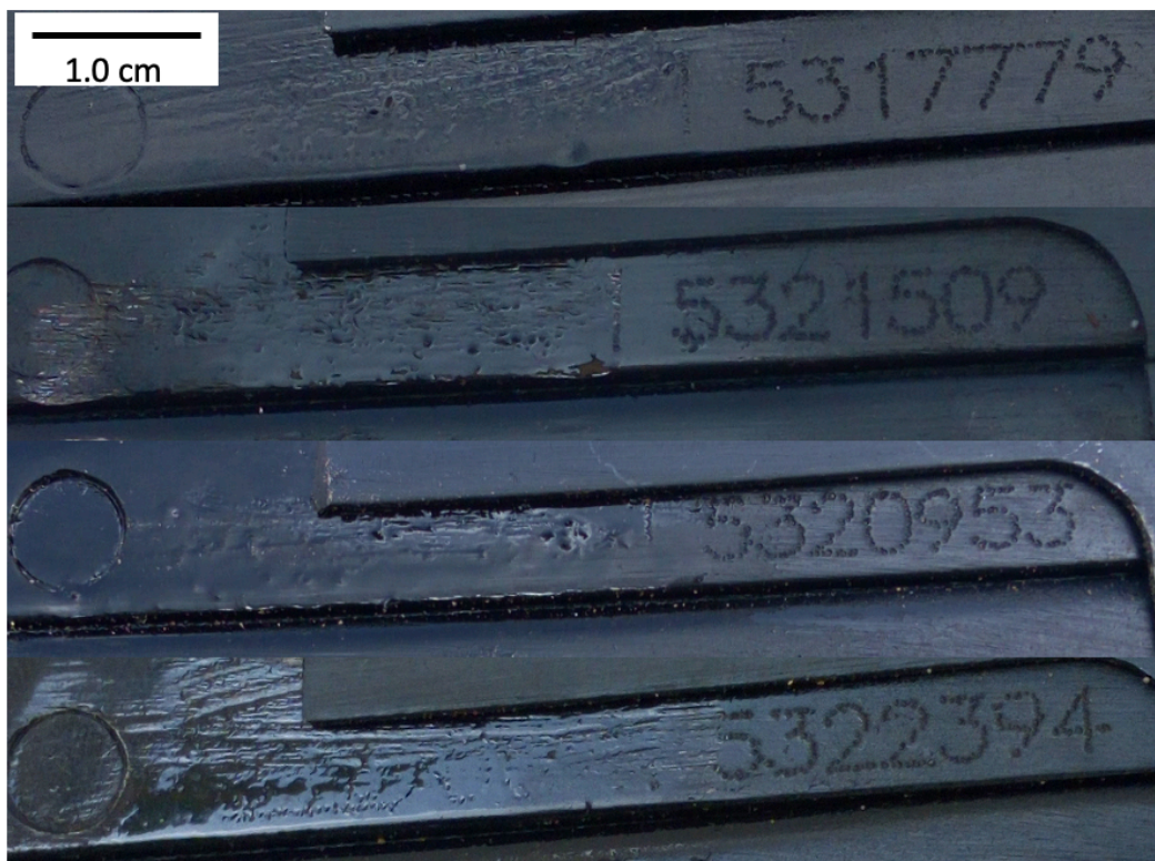
Figure 5: Four examples of weapons with the obliteration code T2.S0.M5/8.D2.C1. The similarity of these weapons may indicate sanitisation by one actor.
