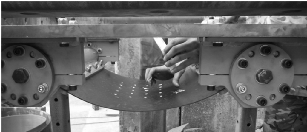
Figure 2. Side view of a target prior to testing, markings on the target were used in conjunction with an oblique high speed video recording to assess the plate deformation during the blast loading.
