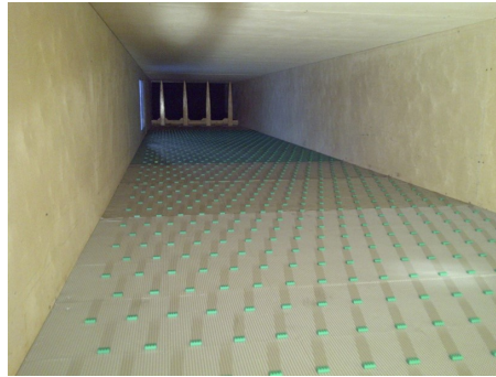
Fig. 8 Setup of the wind tunnel for simulating the Cranfield ABL.
