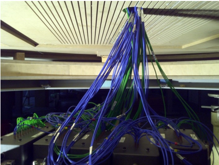
Fig. 11 Tubes from pressure taps fitted on to the transducers located under the turntable.
