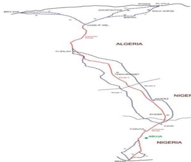
Figure 2-6 Trans-Saharan Gas Pipeline route[26]
