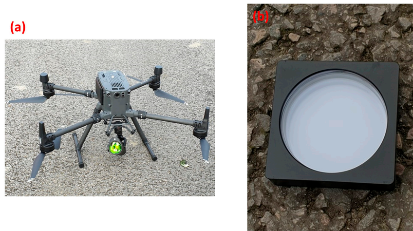
Figure 2. Equipment used. (a) Matrice 300 RTK DJI UAV (DJI, Shenzhen, China) equipped with the U10 sensor. (b) Calibration cell unit; a standard gas sample of \text{CH}_4 of 1700 ppm·m \pm 10%.
