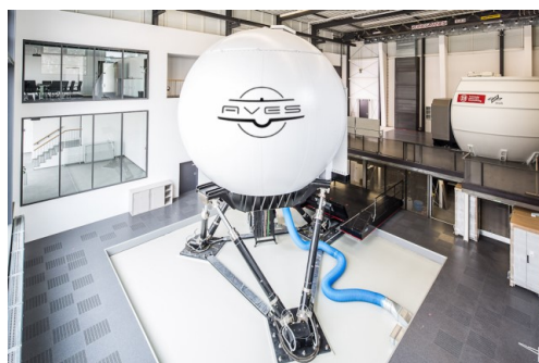
Fig. 1. The DLR AVES flight simulator.
