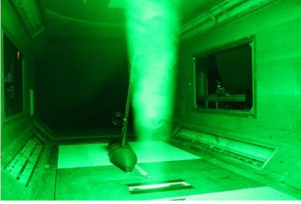
Fig 3 : SPIV laser illumination sheet depicted, from downstream
