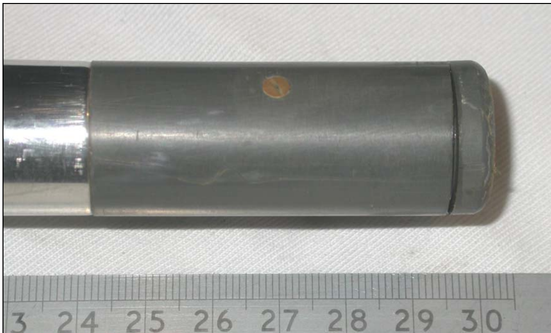
Figure 9A-4: Ex field after 3 years profiling/verification use; splitting of probe tip end seal revealing the internal manufacturing 'O' ring seal
