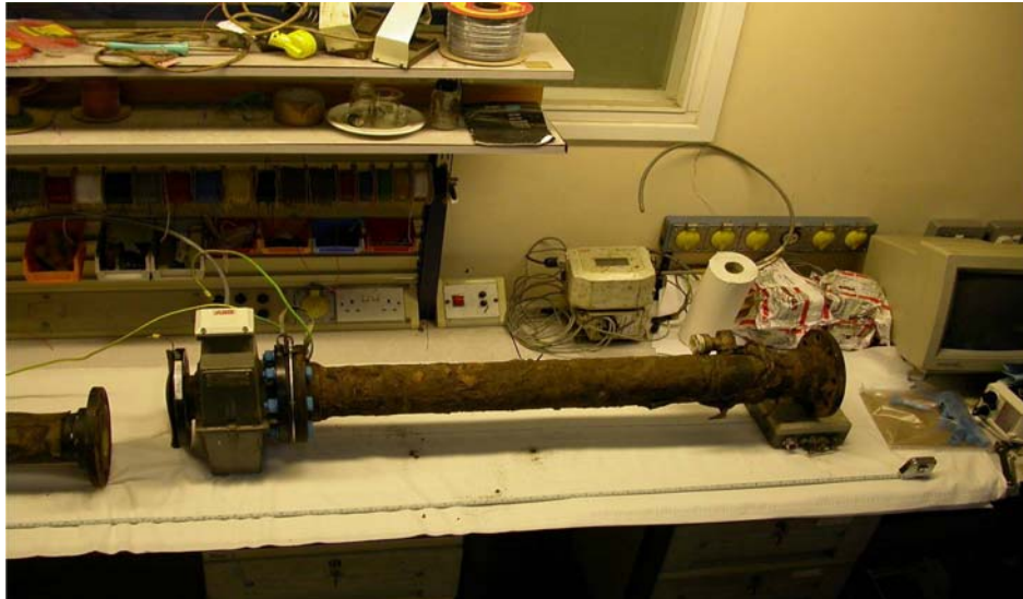
Figure 7.11: Unburied 6yr old SAM metering section - split and with protective tape removed
