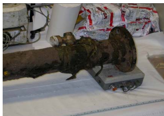
Figure 7.14: Pressure tapping on end of metering section
