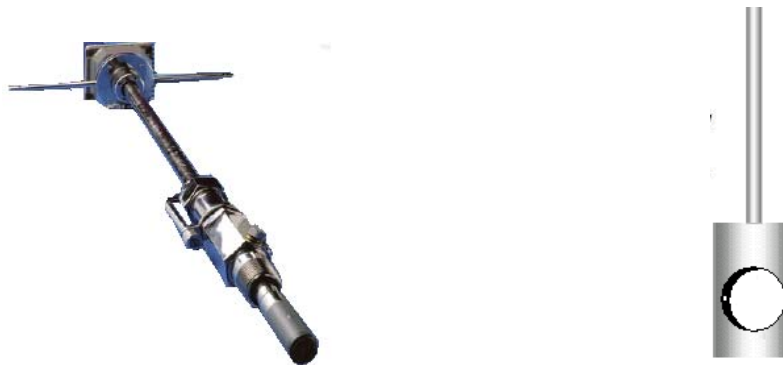
Figure 2.6: Two designs of insertion electromagnetic probes
