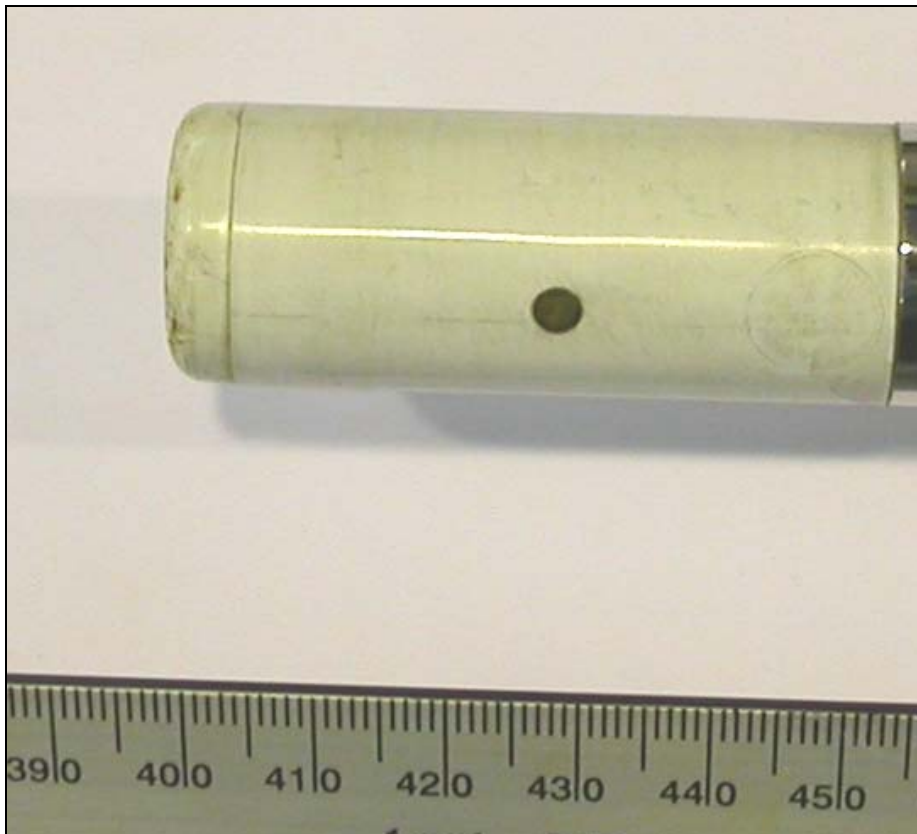
Figure 19A-2: Ex field after 6months profiling/verification use; note change to the geometry of the tip end with flattening of the radial curvature
