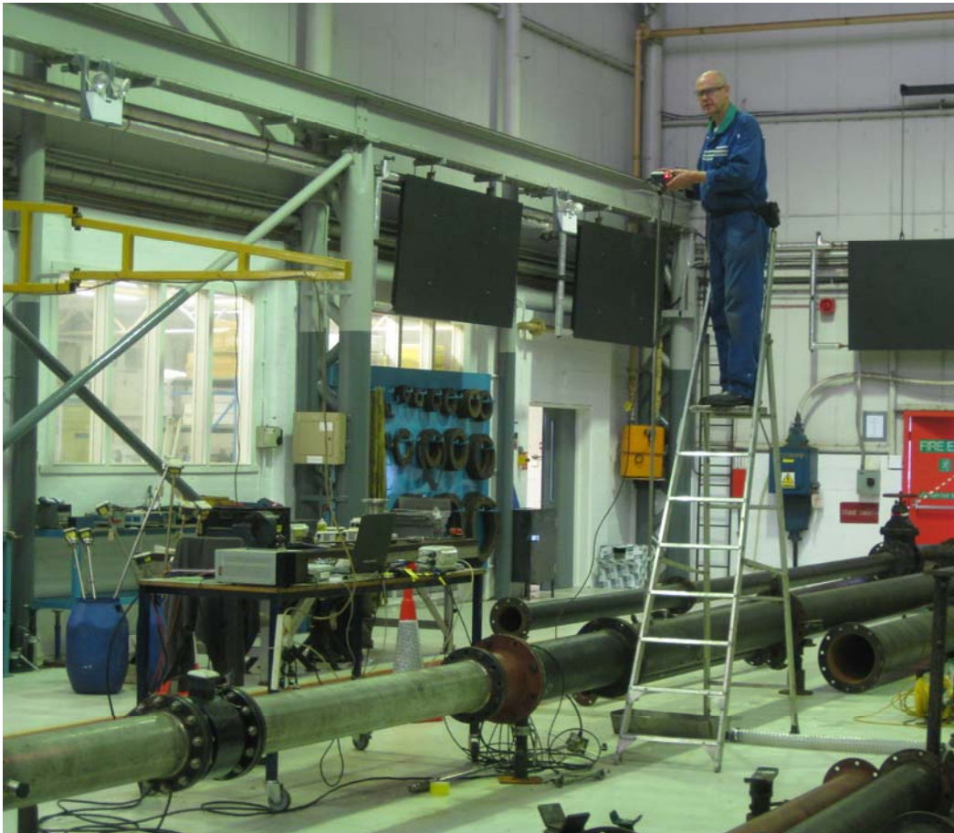
Figure 5.34: Recalibration of 2m battery insertion probe
