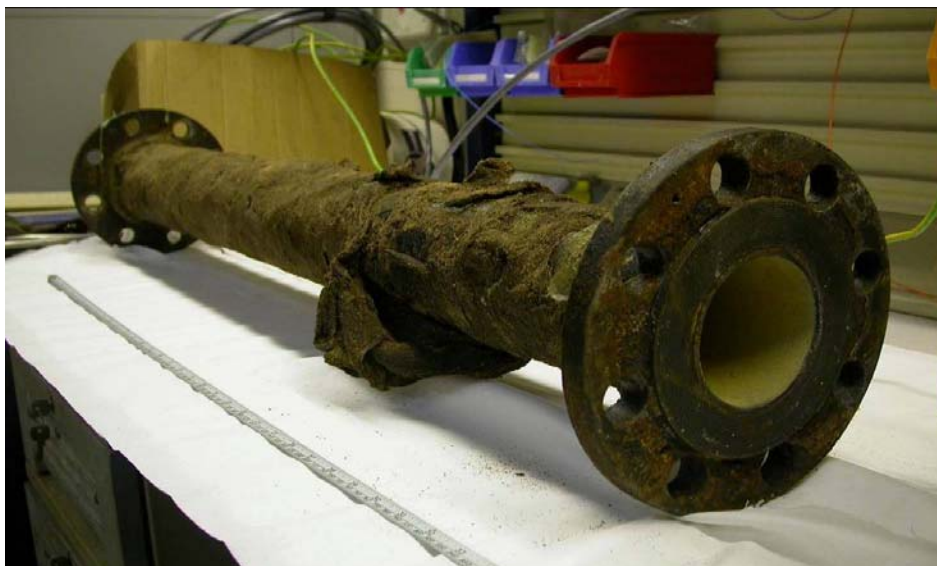
Figure 7.12: Second half of metering section – showing smooth internal bore
