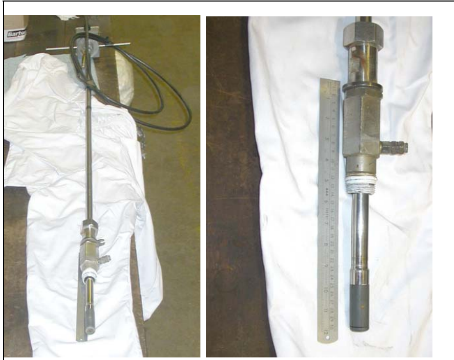
Figure 3.7: 1000mm battery EFM insertion probe assembly
