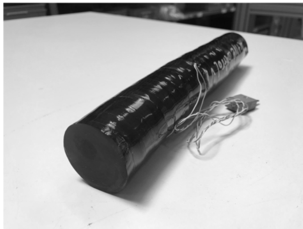
Figure 10 Round cable after the completion of curing stage
