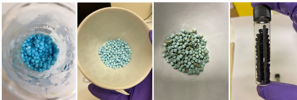
Figure 3-2 Pictures of the \text{Ni}_3\text{Cu}_1/\text{Al}_2\text{O}_3 catalyst (from left to right: after impregnation, after overnight drying, after calcination, and after reduction).
