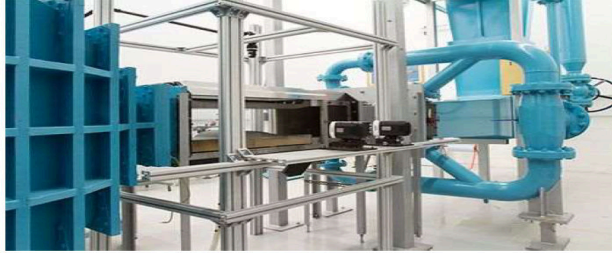
Fig. 1 Transonic Wind Tunnel with model mounted at City University of London, UK.
