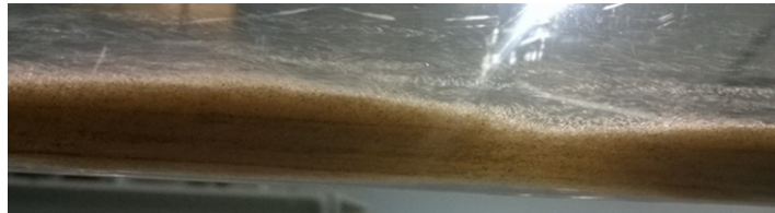
Figure 5.1: Sand bed for 200microns at bottom of pipe ( V_{sl} = 0.1208\text{m/s} ).
