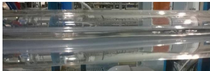
Figure 4.1: Stratified-Smooth Flow from 2-inch flow Pipe (Side View)
