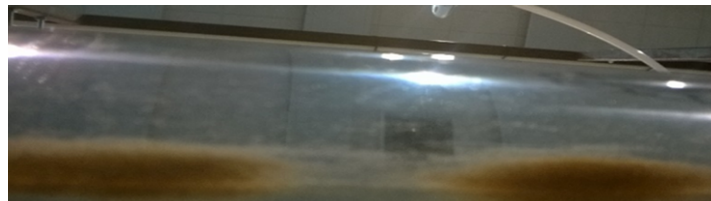
Figure 5.2: Moving dune at bottom of pipe ( V_{sl} = 0.1910\text{m/s} )
