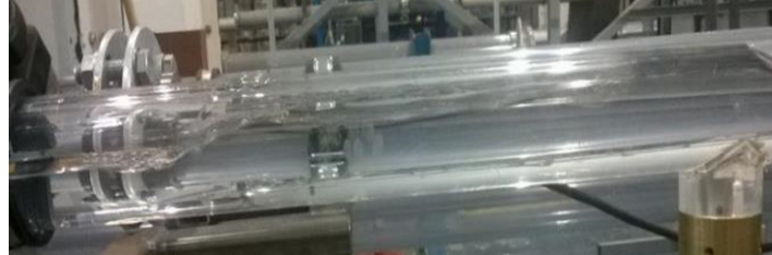
Figure 4.2: Plug Flow from the 2-inch Flow test rig
