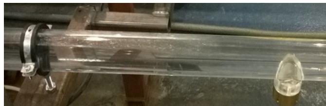
Figure 4.3: Slug Flow from the Experiment using 2-inch Pipe
