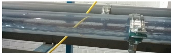
Figure 4.4: Stratified-Wavy Flow from the Experiment using 2-inch Pipe.
