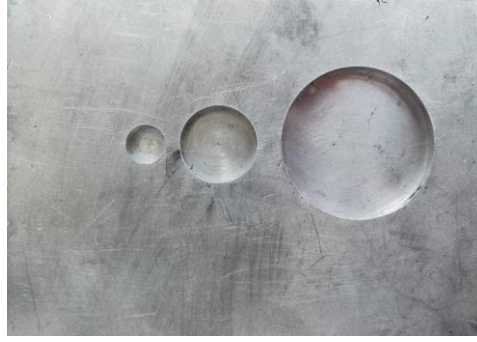
Fig. 4. The drilled surface of the flat-bottom hole samples.
