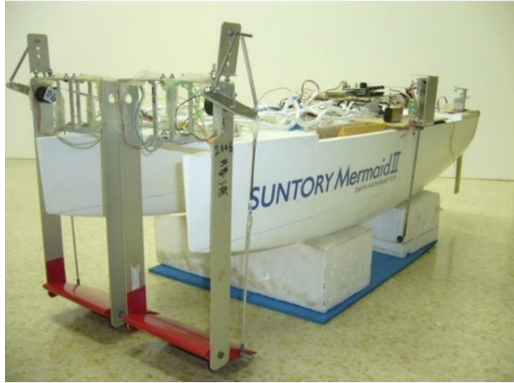
Figure 2.14: Test model of Suntory Mermaid II equipped with all sensors and WDPS (Terao (78)).
