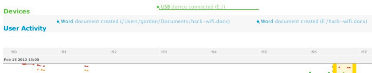
Figure 4. Timeflow visualisation of three events: creation of hack-wifi.docx on local drive, connection of USB, and creation of hack-wifi.docx on E: drive
