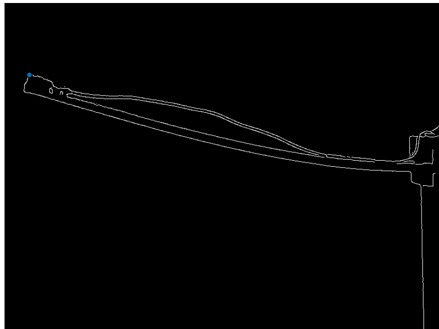
Figure 11. Beam tip detection in the edge image.
