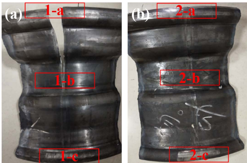
Fig. 17 Wheel rims produced with and without cracking: (a) Sample 1#; (b) Sample 2#.
