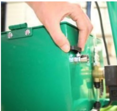
Figure B.12 Air discharge valve located in the front of the SAD
