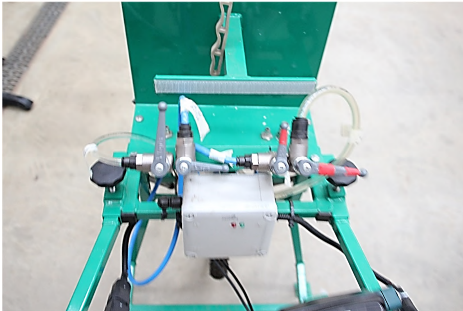
Figure B.10 shows the water (blue) and PAM (red) control valves mounted on the front of the pedestrian sprayer. These control the flow of water and PAM from and to the bottles to the nozzles.
