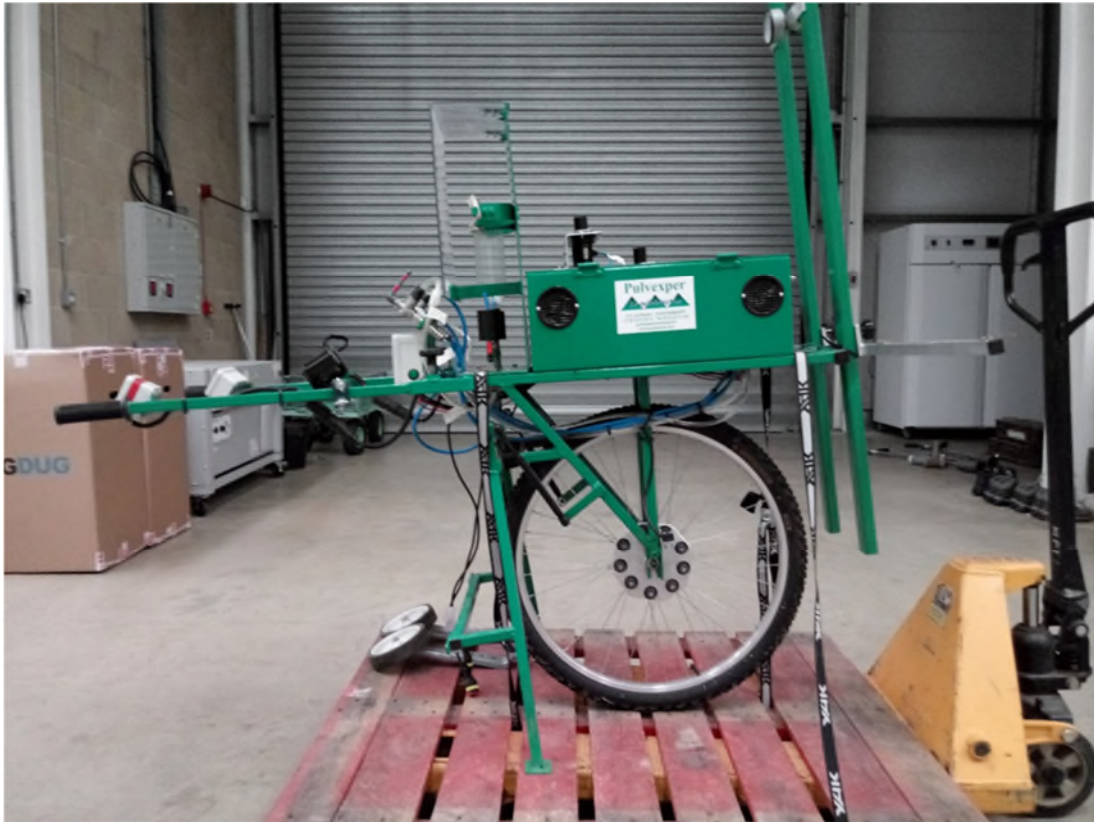
Figure 3.6 Pedestrian Sprayer The main body of the sprayer houses a pressure air chamber that feeds two separate hydraulic systems, for water and polymer. The two feeding systems are regulated independently by two pressure valves located just outside the main body of the sprayer. Detailed SOP available in Appendix B.
