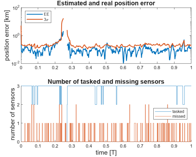
Fig. 6. Tracking using Random strategy and the standard constellation and target parameters listed in Section 2.1. Above, the evolution through time of the target position estimation error (blue) and of three times the RMSE (orange). Below, the number of tasked sensors (blue) and the number of tasked sensors missing their targets (orange) at each timestep.
