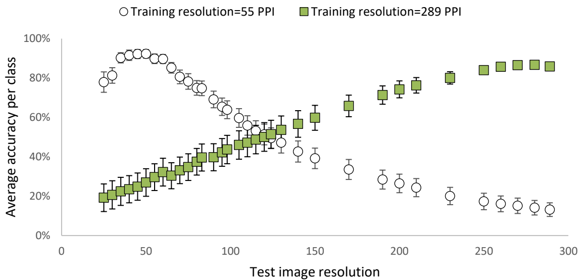
Figure 5-1 – Average accuracy per class for images of different resolutions classified with 2 different networks, one trained with 55 and the other with 289 PPI images. Vertical bars show the standard error for each tested resolution.
