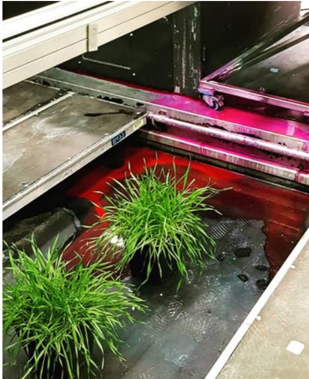
Figure 2-5: Pots of Winter Wheat under the track sprayer at Silsoe Spray Application Unit Ltds, Bedfordshire.
