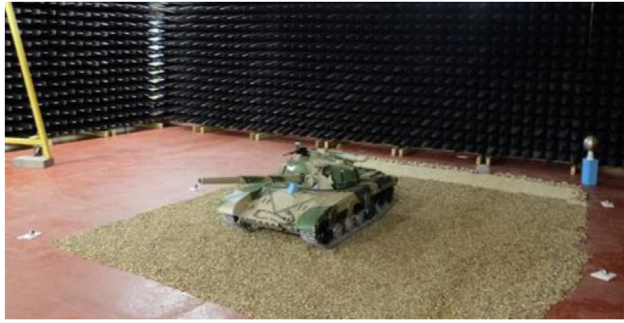
Fig. 3 The measured scene, consisting of the quarter-scale model tank on gravel.
