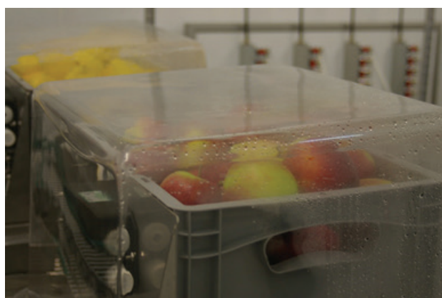
Fig. 2. LabPod (Storage Control Inc, USA) storing Gala apples
