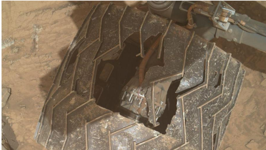
Figure 2-1 Wheel damage on the Mars Curiosity Rover (BBC Newsround, 2024)
