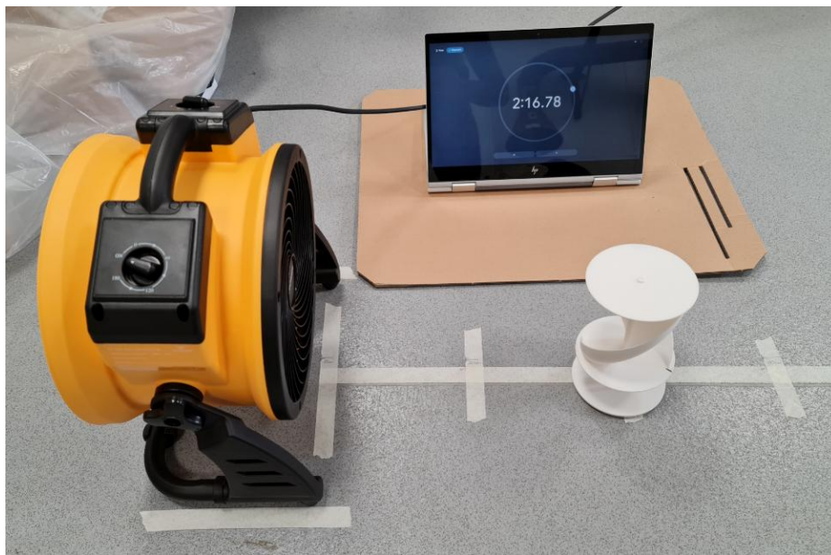
Figure 6-6 Experimental set-up for turbine performance testing
