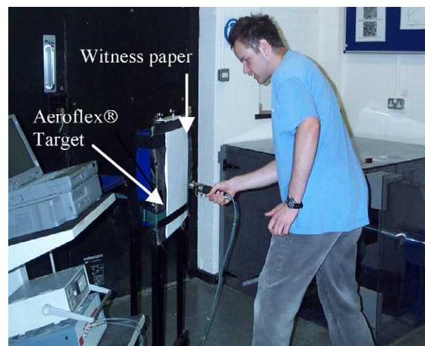
Fig. 1 Volunteer slashing a vertical target with an instrumented blade.
