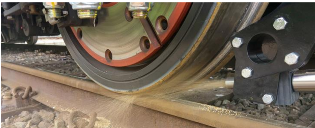
Figure 3-10 Wheel-rail contact with a sanding system (Ricardo, 2019).
