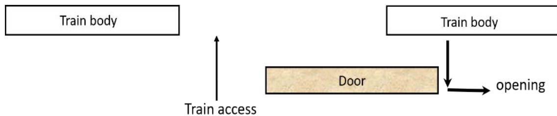
Figure 3-3 Sliding Plug Door Motion.
