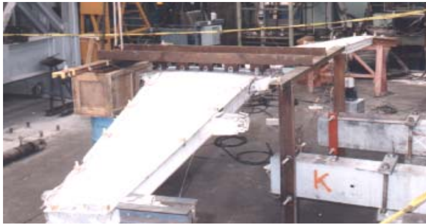
Figure 1. A view of the tail-plane set-up for vibration test
