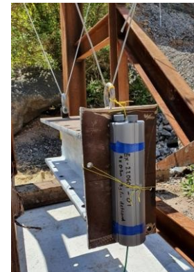
Fig. 1c. "V" suspension reduced torsional rotation
