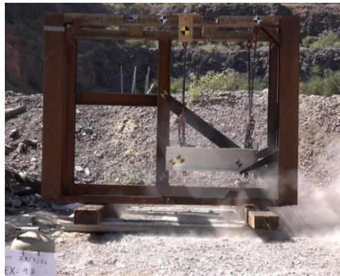
Fig. 1b. Test apparatus with medium mass (122kg)
