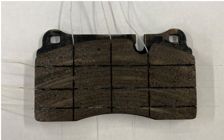
(b) FM Surface after Dynamic Tests
