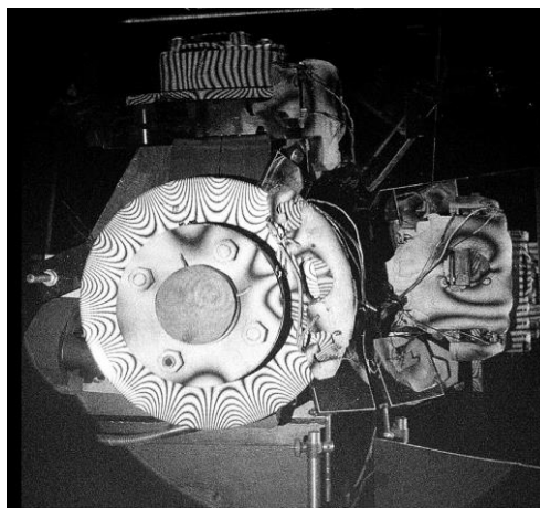
Figure 2-15: Photograph of Mode Shapes Using Laser Holographic Interferometry (Fieldhouse, 2013)
