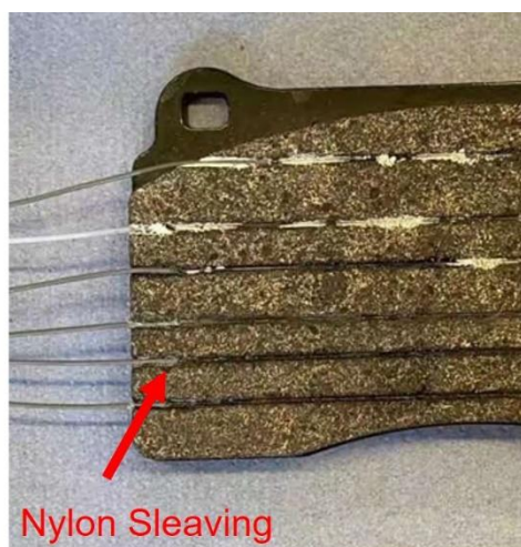
(b) Installed FBG Sensors at The Horizontal (X) Direction
