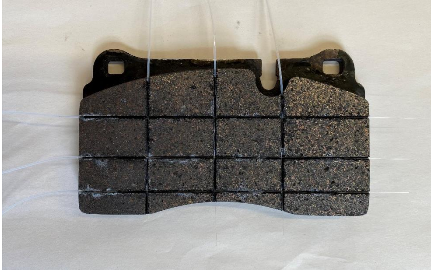
(a) FM Surface before Dynamic Tests
