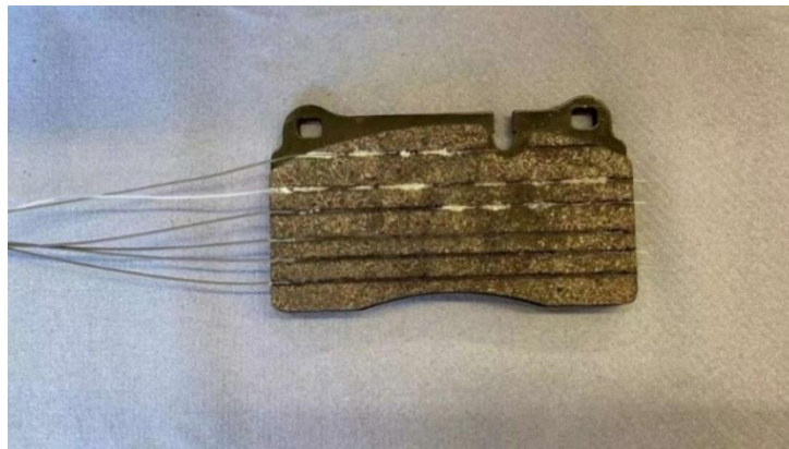
(b) Installed FBG Sensors at The Horizontal (X) Direction
