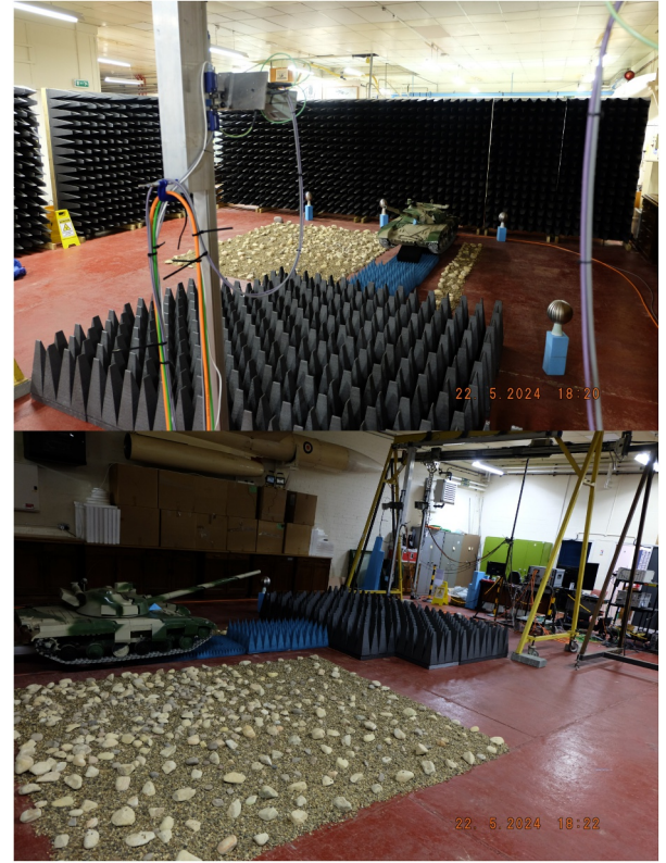
FIGURE 6 | Experimental setup looking downrange of GBSAR system (above) and across/up-range (below).
