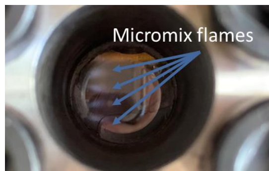
Figure 7- Optical access window to observe hydrogen micromix combustion.
