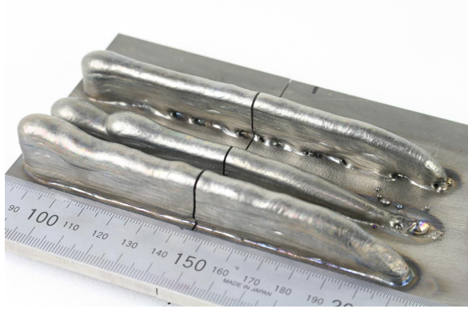
Figure 4: Examples of Ti-6Al-4V walls build by Plasma Wire Deposition (main ruler unit is cm).
