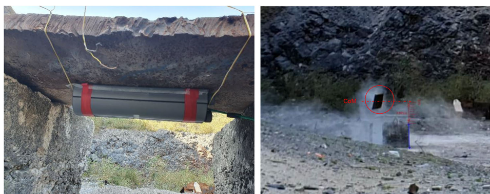
FIGURE 1 | (a) Charge positioned on underside of steel plate, (b) Steel plate projected vertically to estimate the impulse from explosive charges.
