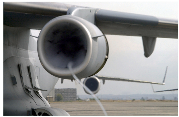
Fig. 6. Tightly-wound ground vortex during taxiing. Source: The U.S. National Archives.
