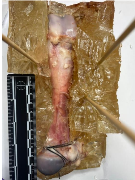
Figure 16: Bone 2/6 during the gelatine removal process. Wooden pointers showing the bullet paths.
