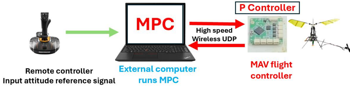
Fig. 16 E-MPC implementation framework on HFWR MAV
