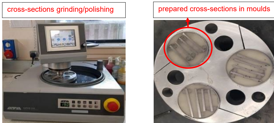
Figure 2 Grinding and polishing of mounts (using SAPHIR 550) to prepare cross-sections of corroded steel samples, for measurement of corrosion depths under DM- image analyser technique
