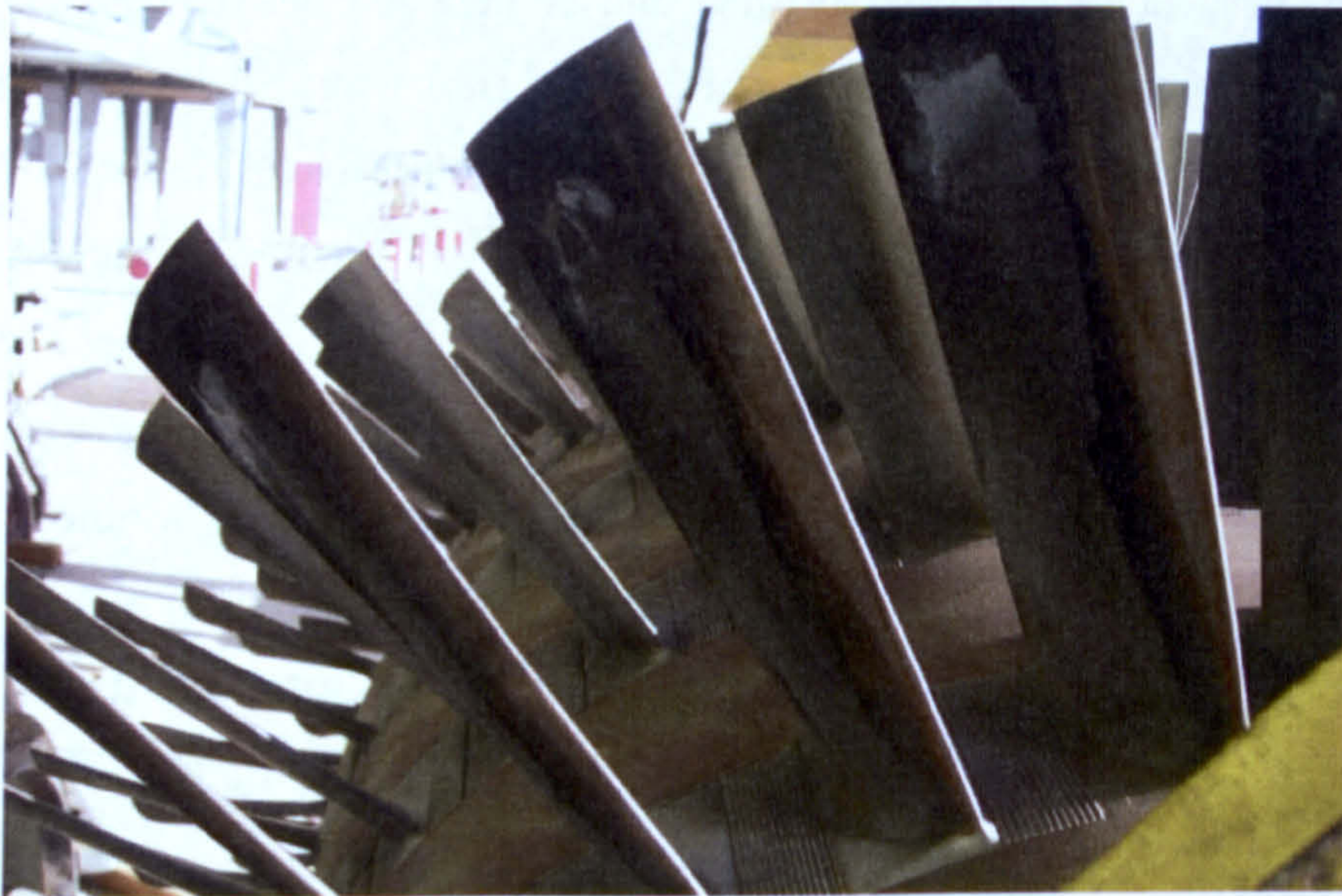
Figure 2-11: Compressor Fouling Due to Erosion in a desert environment (Courtesy of ENI Oil – Libyan branch, Abu-Attifel Field, 2008)
