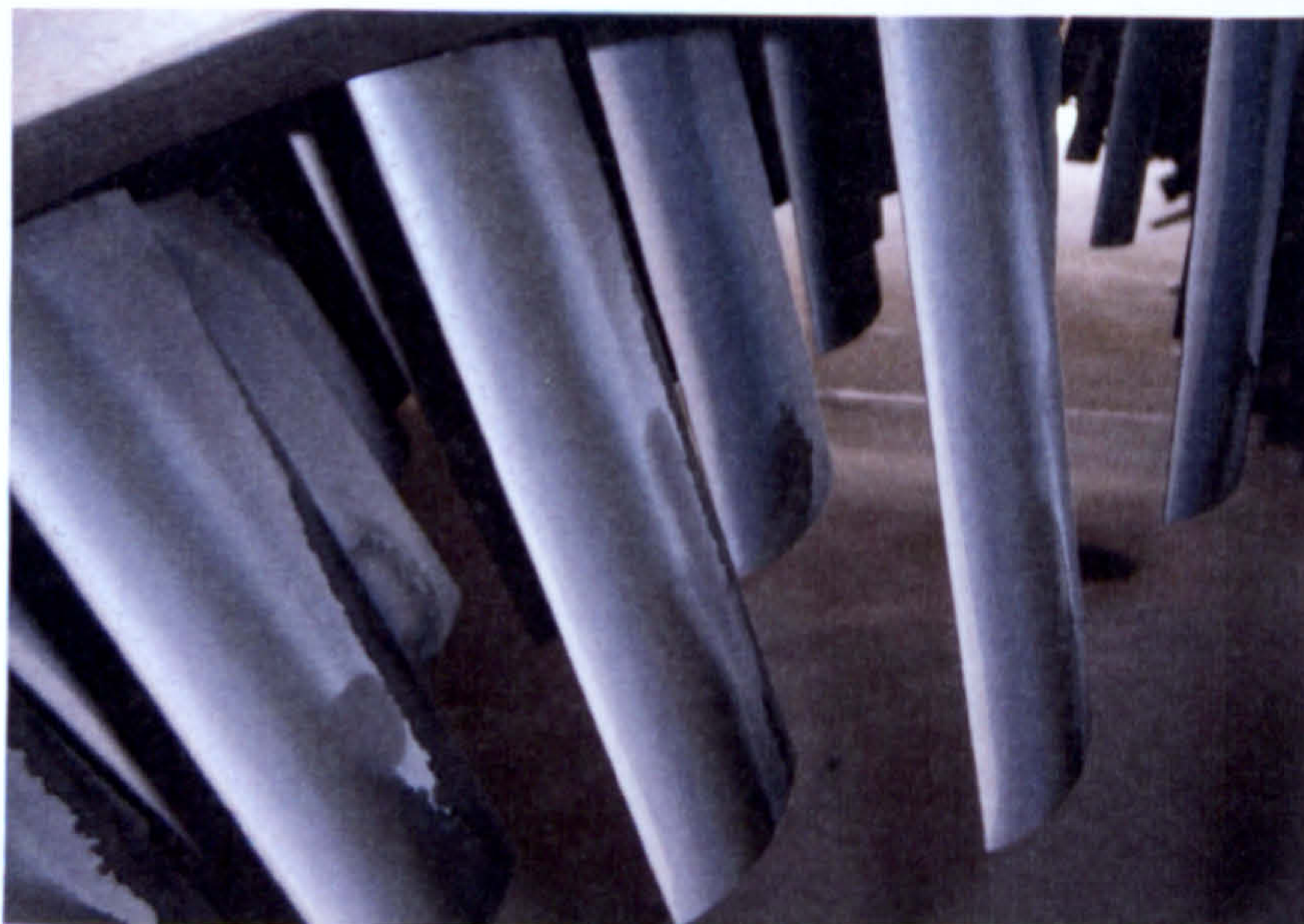
Figure 2-4: Compressor stator blades fouling of Sulzer type 7 (Courtesy of ENI Oil – Libyan branch, Abu-Attifel Field, 2008)
