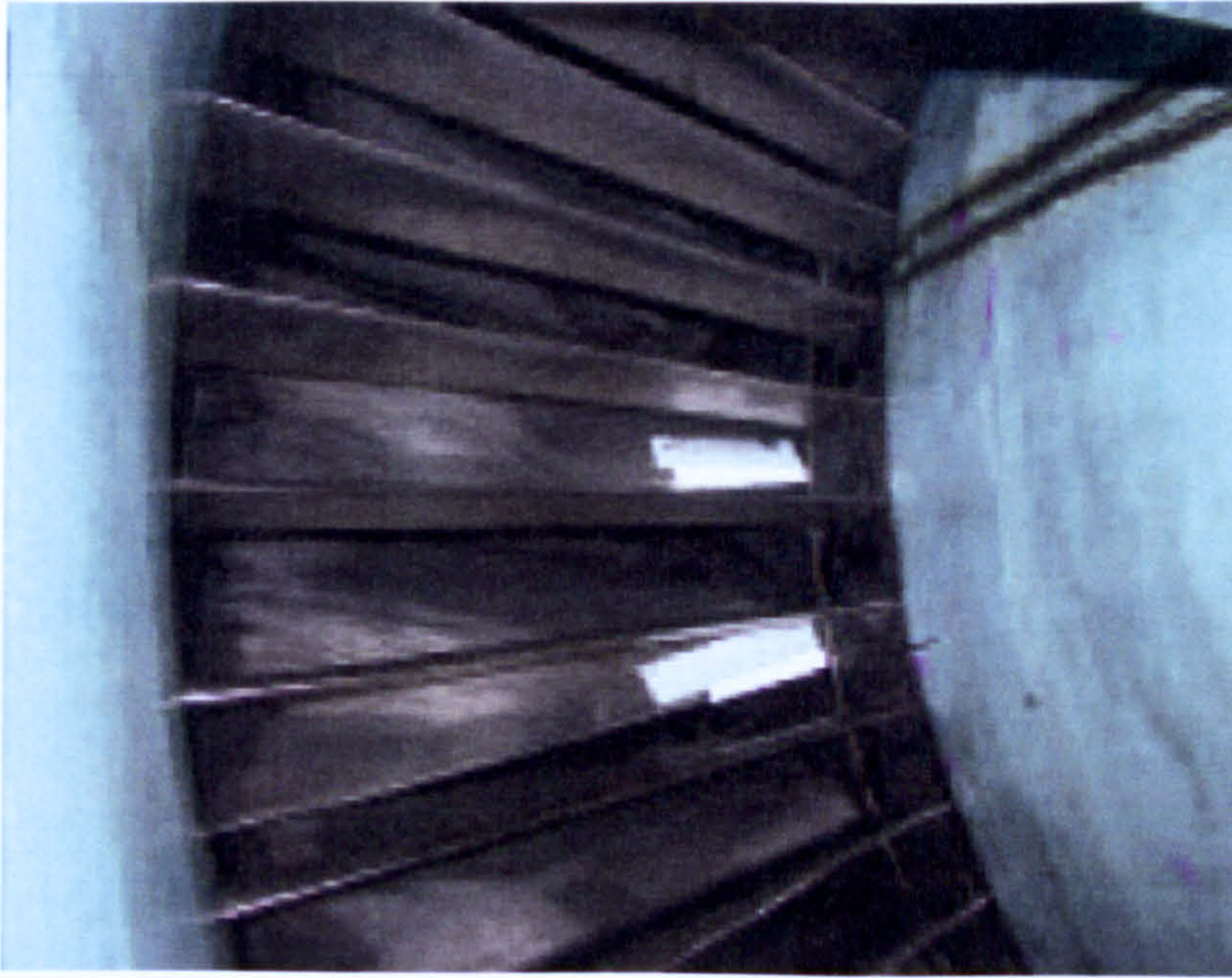
Figure 2-9: Molds applied on leading edge of R0, 1 st stage, compressor blades on Unit EC-6 (Oosting, J. and Stalder, J. P., 2007)
