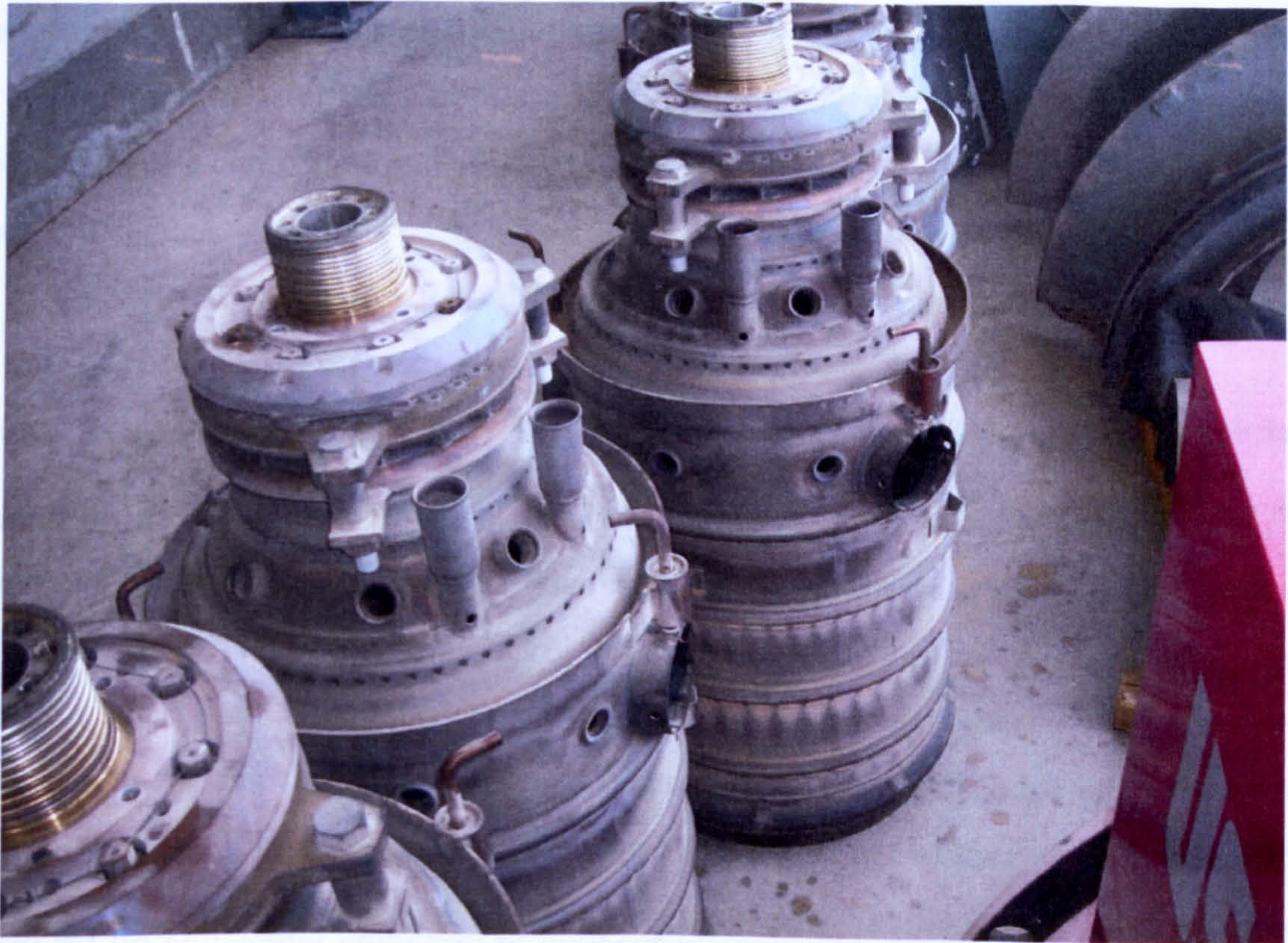
Figure 3-6: Combustion Chambers (Courtesy of ENI Oil – Libyan branch, Abu-Attifel Field, 2008)
