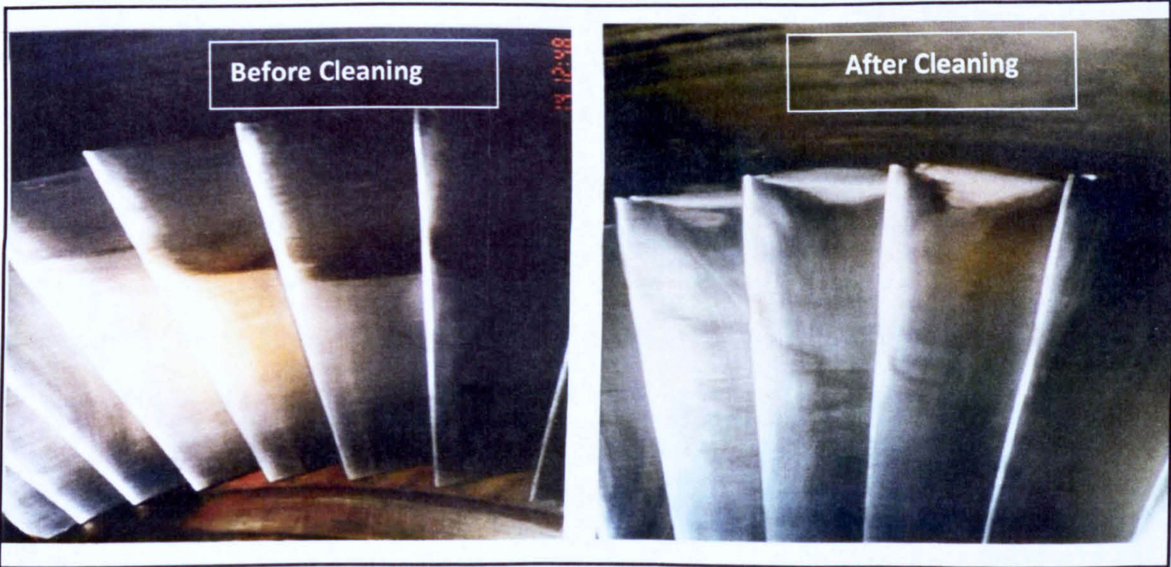
Figure 2-37: Compressor Blades before and after Cleaning (Haub B. L., 1990),
