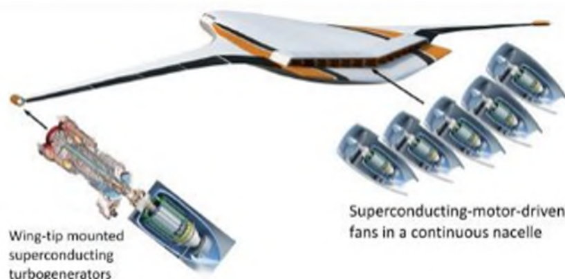
Figure 2-5 N3-X aircraft TeDP concept
