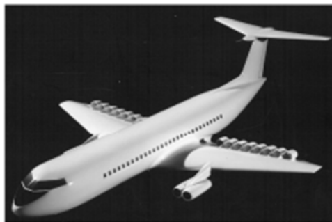
Figure 2-3 STOL transport using LPC discharge tip-driven multi-fans [9]
