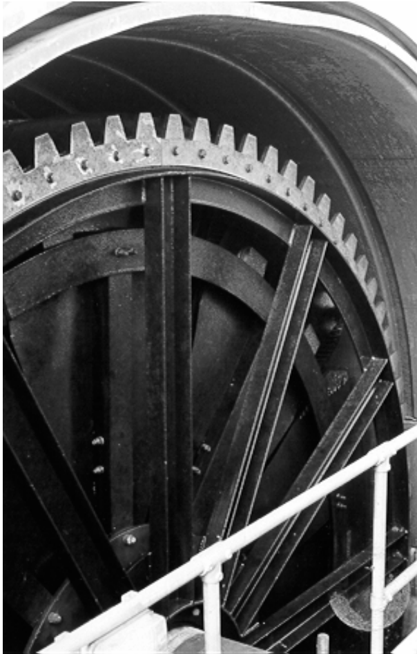
Figure 87 (left) Pinion and gear transmission arrangement; Larger gear wheel
