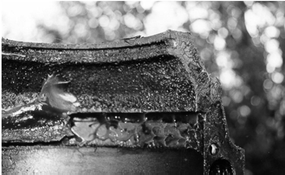
Figure 97 Evidence of rust in a bearing housing
