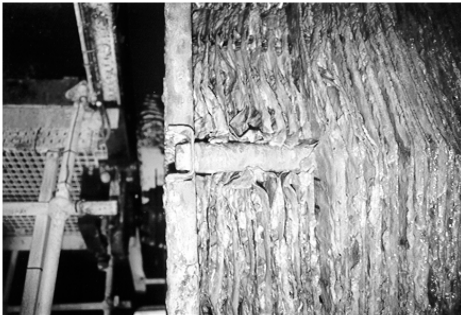
Figure 24 Tearing of High density polypropylene media panels in the vicinity of the support through rod
