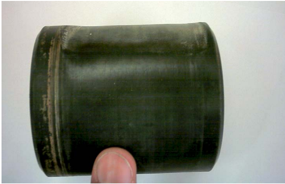
Figure 92 Evidence of uneven wear due to misalignment
