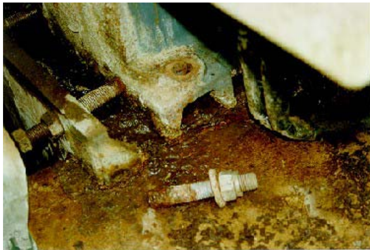
Figure 40 Fracture of foundation bolts due to transient torque produced by loose media pack
