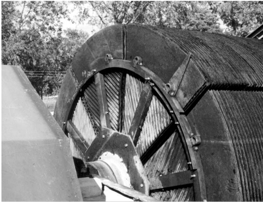
Figure 30 Design to overcome loss of rigidity
