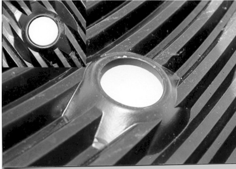
Figure 29 Improved strength of hole in media panel
