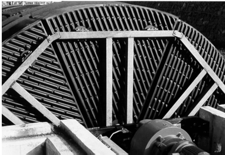
Figure 54 RBC design arrangement showing double radial spider arms per media segment
