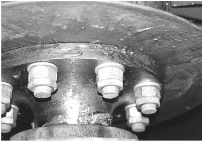
Figure 76 Improper bolting of double lock nuts
