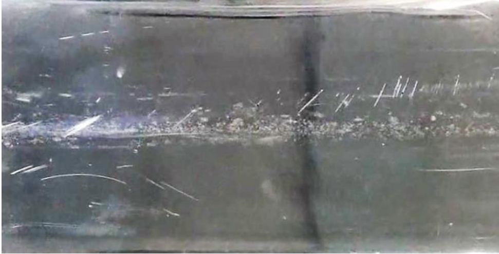
Figure 5-17: Snapshot of sand streak below MTC, (200lb/1000bbl, 212 microns V_{sl}=0.06\text{m/s} , V_{sg}=3.9\text{m/s} , Flow: left to right, View: Bottom)
