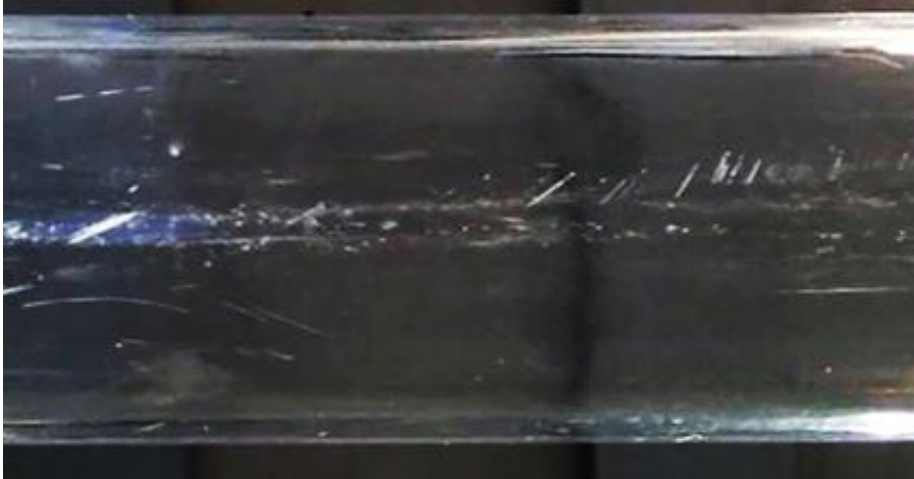
Figure 5-15: Snapshot of sand streak at MTC, (200lb/1000bbl, 212 microns V_{sl}=0.06\text{m/s} , V_{sg}= 4.1\text{m/s} . Flow: left to right, View: Bottom)
