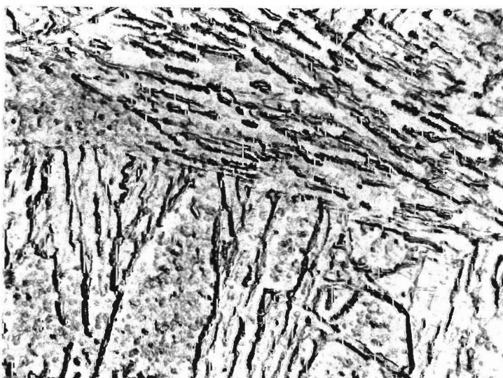
Figure 28. Microstructure produced by double thermal cycling to a peak temperature of 1275°C. Carbon extraction replicas.
