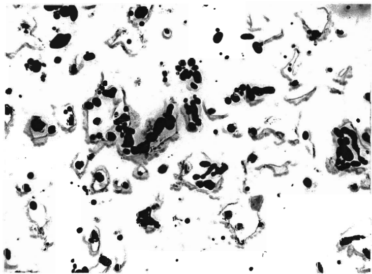
Figure 33. Microstructure produced by double thermal cycling: initial and second peak temperatures of 930°C and 765°C respectively. Carbon extraction replicas.
