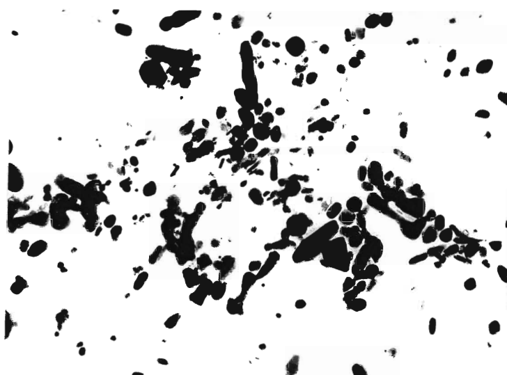
Figure 41. Post cycle heat treated microstructure of the double thermal cycled 930/765°C peak temperature condition. Carbon extraction replicas.
