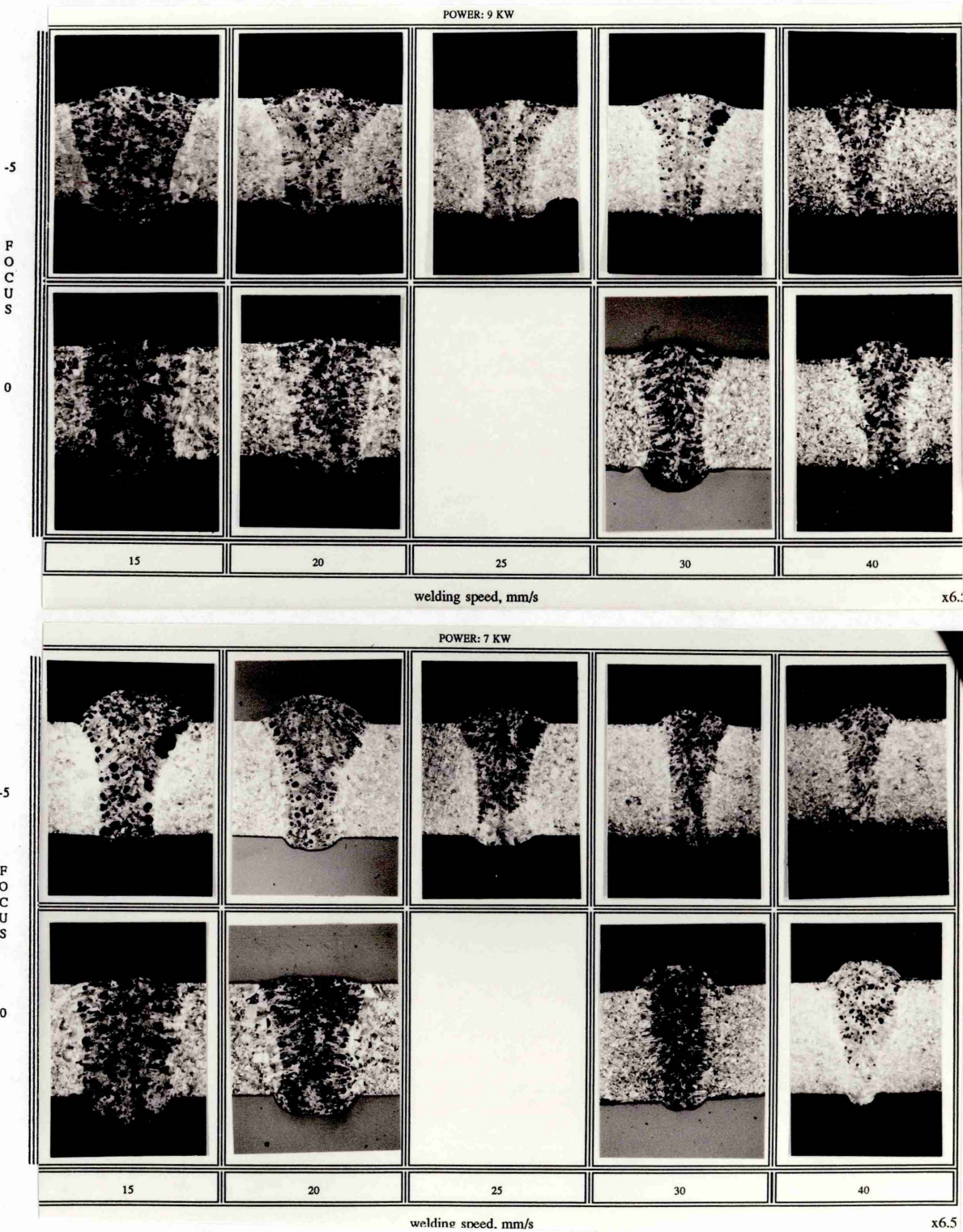
Fig. 4.8 - Influence of beam power, focal position and welding speed on weld bead profiles
