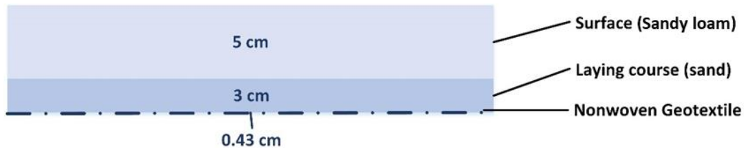
Figure 1-6 Cross-section of three layers structure for simulating the hydraulic performance of soil, sand and geotextile
