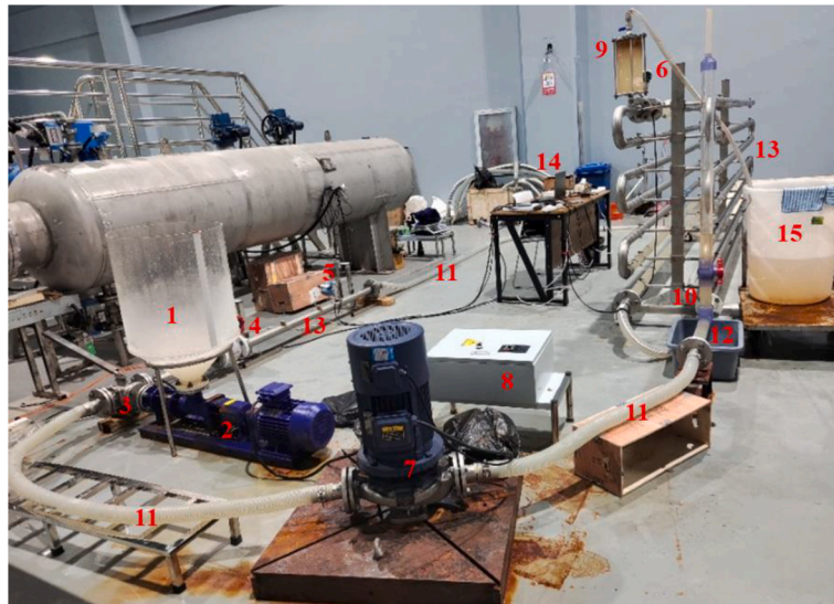
(a) Experimental rig setting: 1. Ice bucket, 2. Screw pump, 3. Three-way valve, 4. Electromagnetic flowmeter, 5. First temperature sensor, 6. Second temperature sensor, 7. Pipe circulating pump, 8. Frequency converter, 9. Water draining device, 10. Air exhausting device, 11. Transparent hose, 12. Transparent plastic pipe, 13. Horizontal symmetrical stainless-steel pipes, 14. DAQ (Data acquisition system), 15. Water discharge bucket
