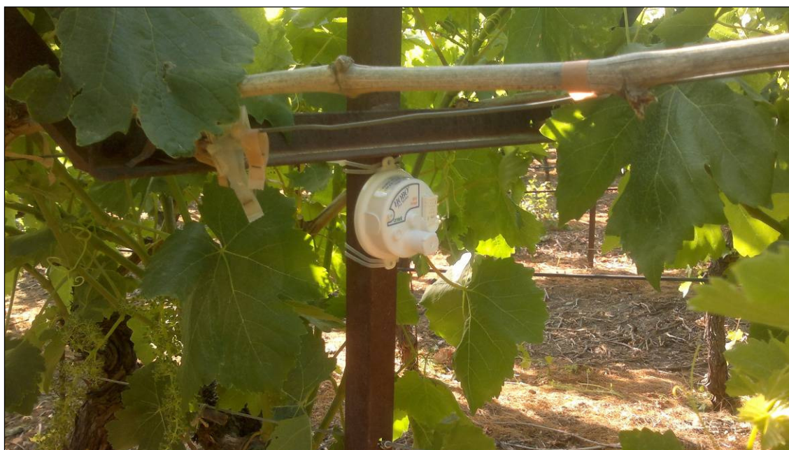
Plate A.2. Temperature and Relative Humidity Data Logger (HOBO – Onset, USA), placed inside the canopy of Soultanina vines, in an experimental vineyard.
